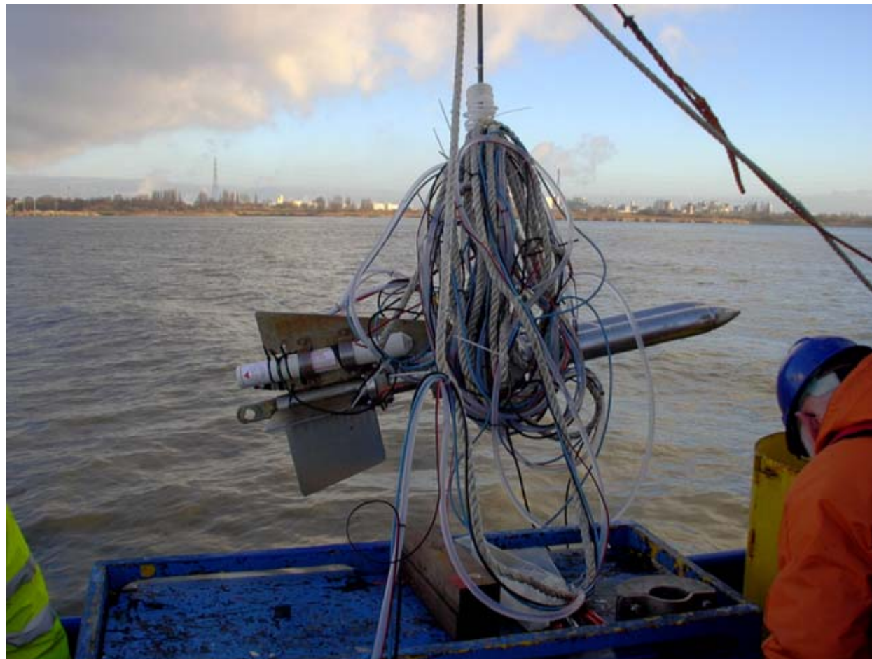
Figure 2-2: Fish mounted with Navitracker density probe, CTD-OBS sensors and watersampler
