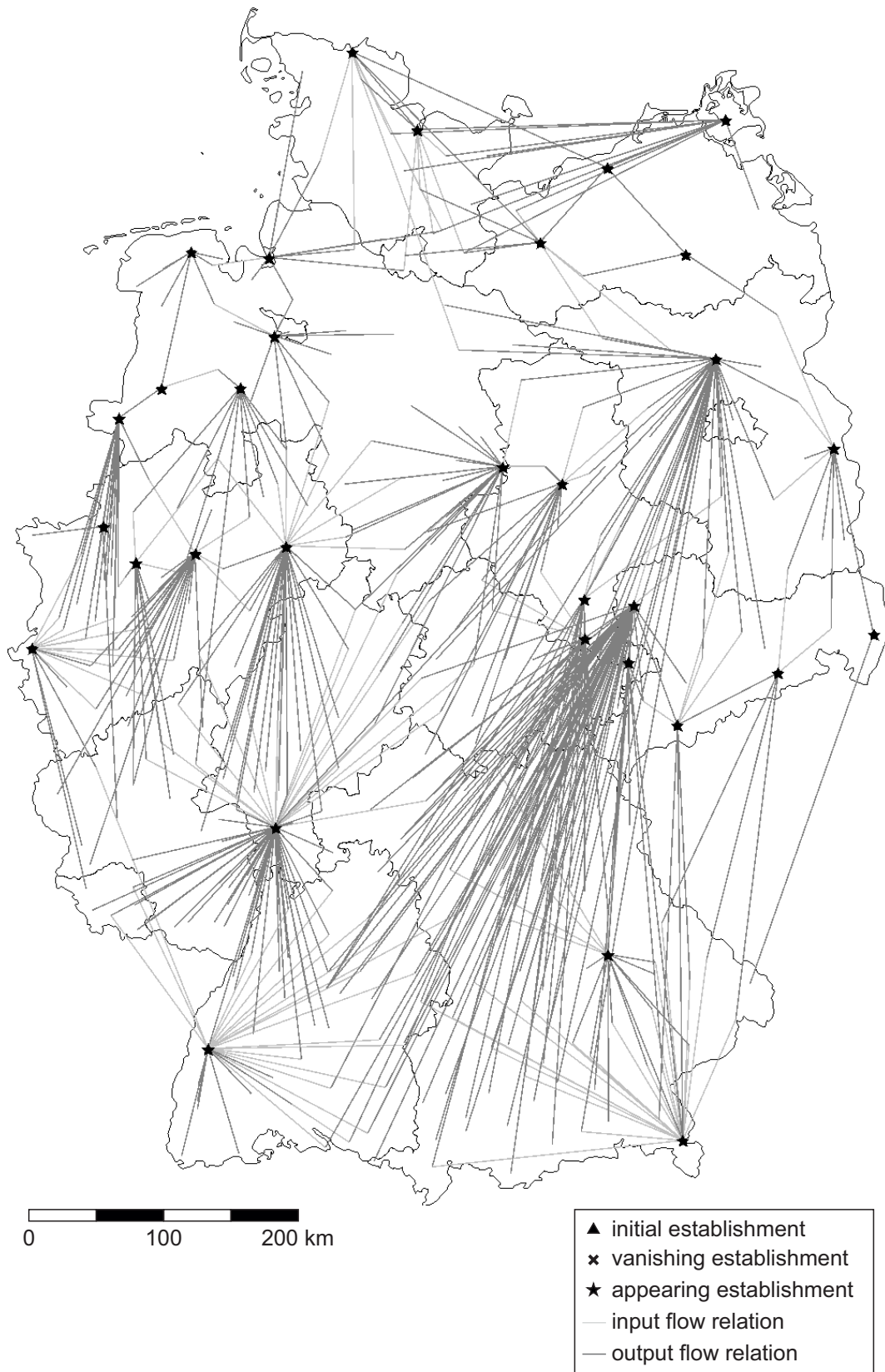
Figure 5.14: Map showing the up to 32 establishments that appear during centralisation of poultry slaughtering if optimal location choice, optimal assignment, and minimisation are assumed ( OptOptMin )
