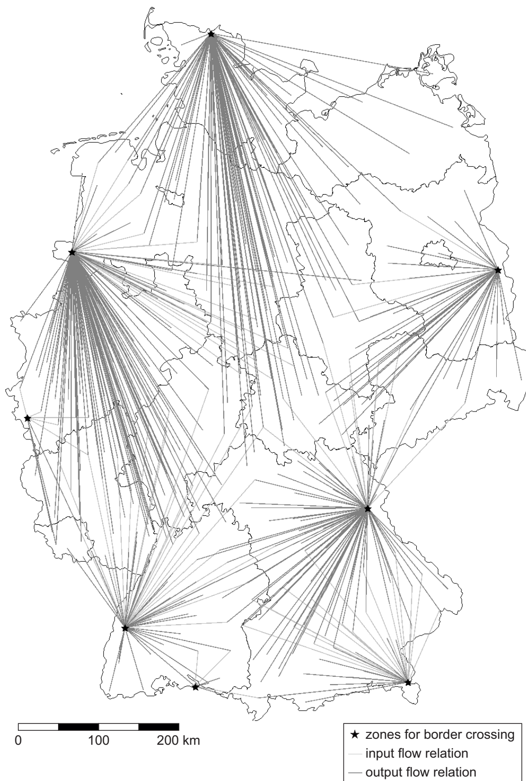
Figure 5.22: Map showing the domestic freight flows resulting from freight transport performance minimisation in the case of complete offshoring of poultry slaughtering (WZ 10.12). Assignment of volumes according to import data in table A.2 (page 206) in appendix.
