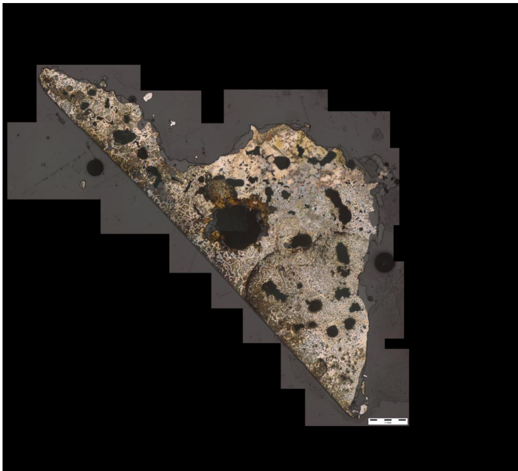
Figure 4.6.2 Composite image showing metallographic sample 2 in the etched condition scale bar 1mm.
