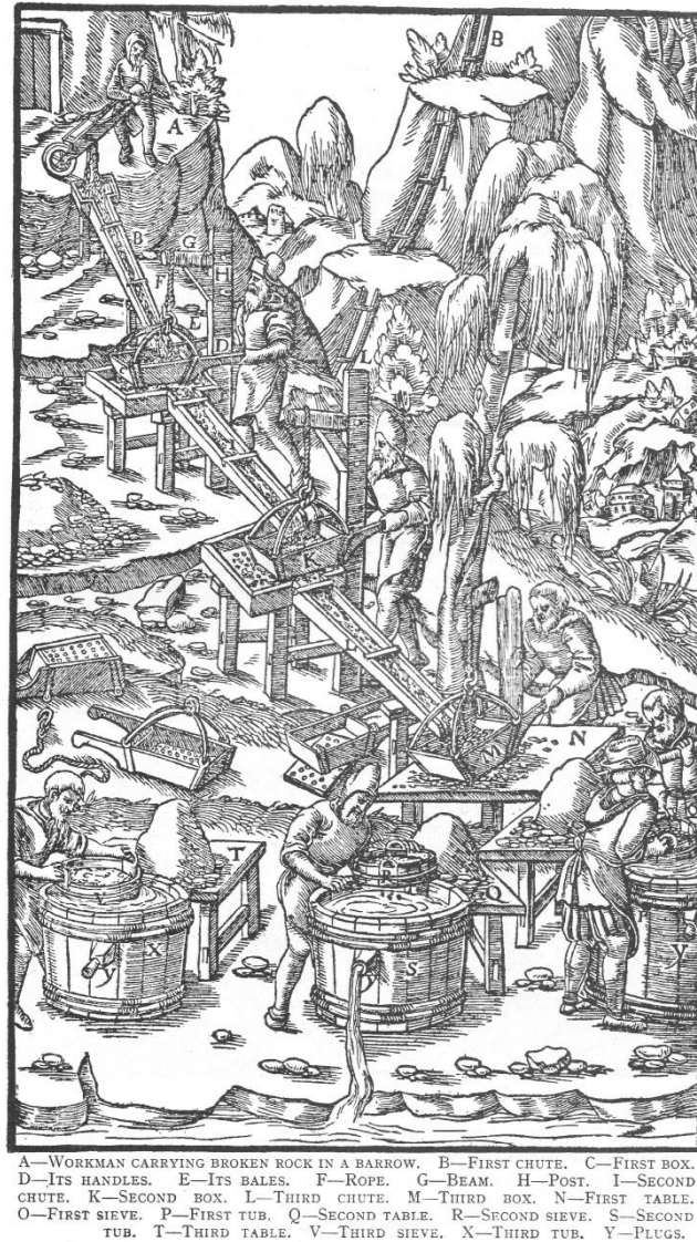
Figure 2.6.2 Showing ore extraction and washing Agricola [1556] (Hoover and Hoover: 291).
