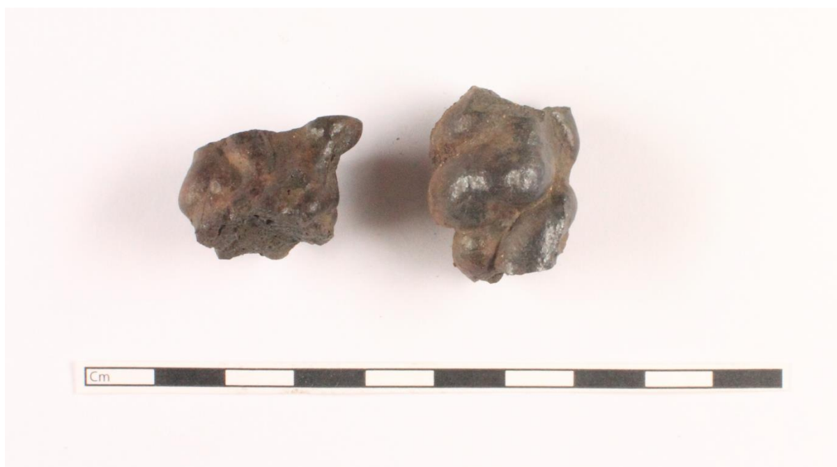
Figure 6.4.5 showing flowed smelting slag from context FLX89 2176 (a and b, left and right respectively).
