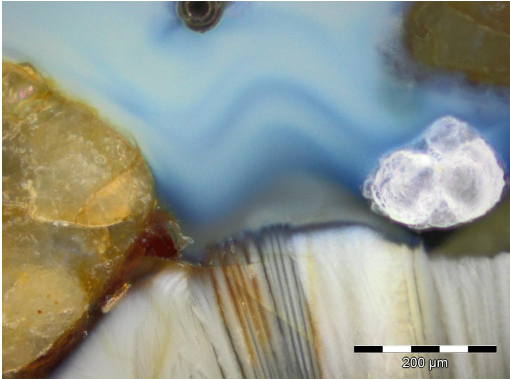
Figure 6.2.16 Showing glassy region with blue colouring with feathered fayalite (white) and silica grains.
