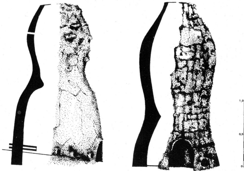
Figure 3.2.2: Showing the difference between the attempted copy (left) and the original induced draught-furnace constructed in 1910 (van der Merwe and Avery 1987: 152).
