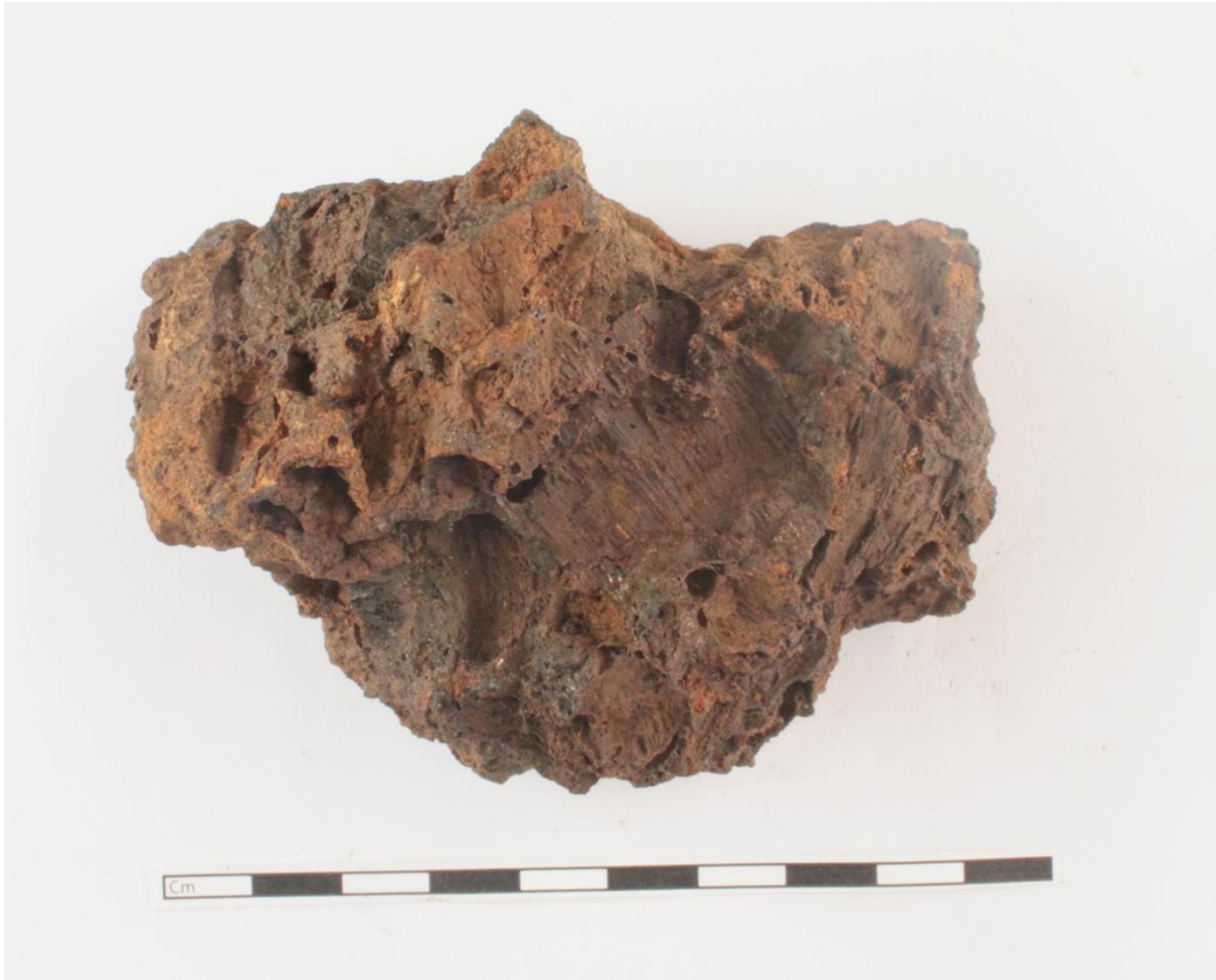
Figure 6.1.3 Hasholme Hall smelting slag with fuel inclusion marks – dark central region and surviving fuel inclusions, black charcoal in circular pore below large fuel inclusion impression.
