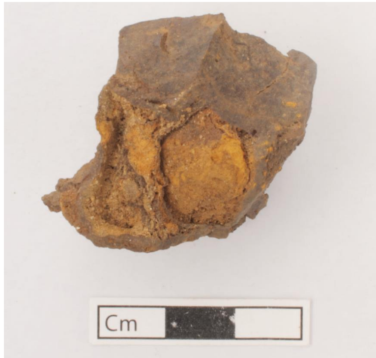
Figure 6.4.18 showing sample of material from FLX89 800 with slag encasing iron- rich stone.
