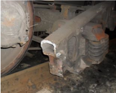
Fig. 1. Typical breakdown of bogie side frames
