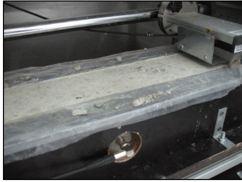
Fig.7: Location of the transmitter of ultrasonic pulse
