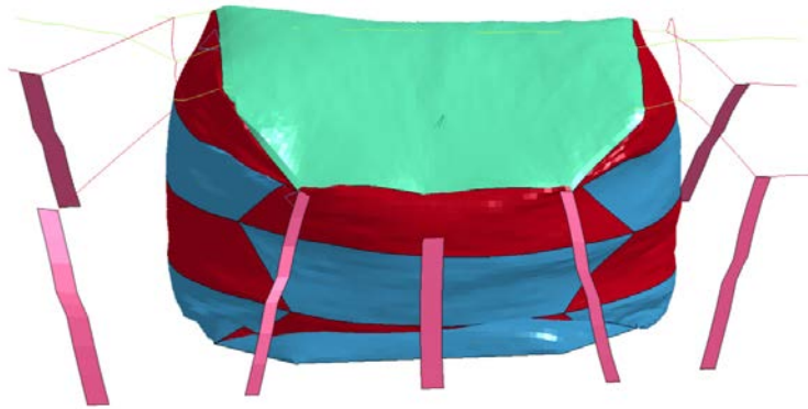
Figure 15 Typical bag design for morphing wing
