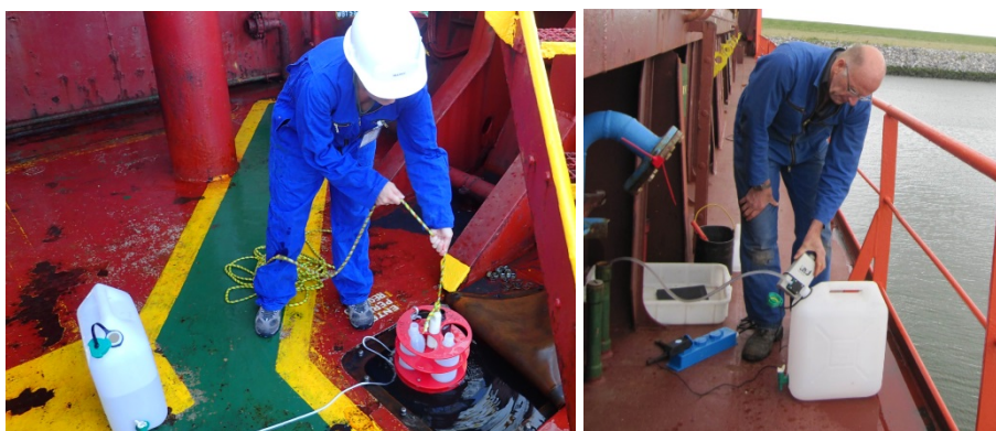
Photo 1. Left: sampling vessel 3 using the carousel in manholes; Right: sampling vessel 1 via air channels.
