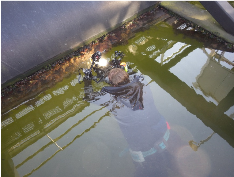
Figure 3. Inventory of floating dock by snorkelling.
