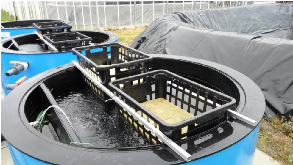
Figure 2: Basin detail, baskets mounted on different heights on aluminium tubes. Shown here are basin 1 (back) and 2 (front), the bubbles from the air supply are clearly visible.
