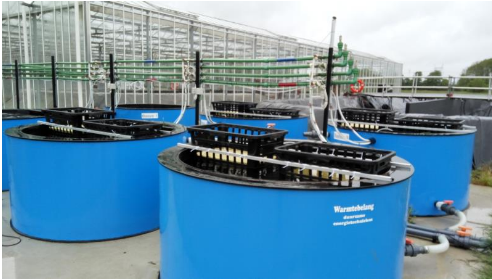
Figure 1: Overview of the experimental setup, the 4 basins in front are used in the experiment. The baskets were lined up in north-south direction. The green piping is used for heat and/or cold supply to regulate the basin temperature.
