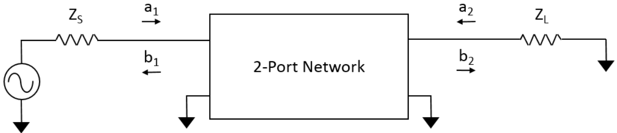
Figure A.2 2-Port Network Model.
