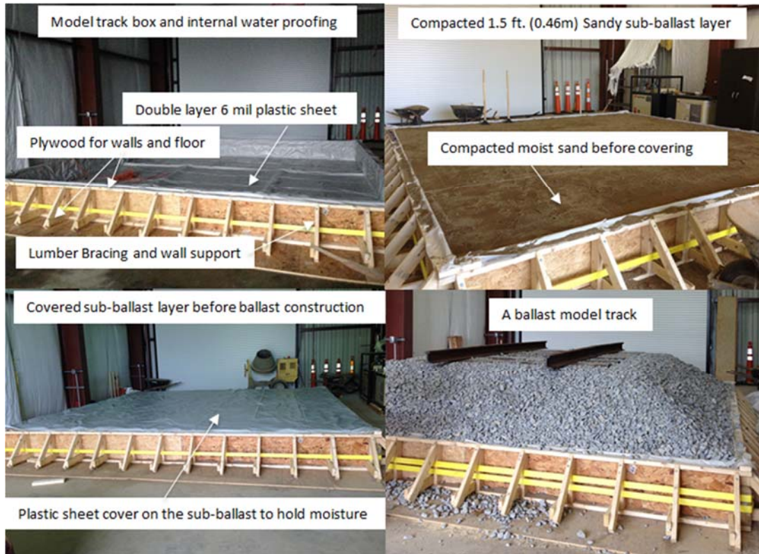
Figure 3.2: Full-Scale Model Construction Process.
