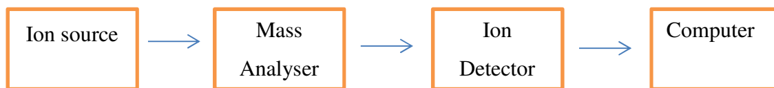
Figure 1.5.1 Schematic of the basic components of a mass spectrometer
