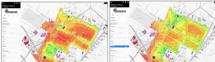
Figure 2. Weighting section on the front interface of InViTo. The maps show the spatial effect of selected criteria depending on assigned weights. The variation of weights on the left side menu makes the map on the right side changing in colours through a traffic-light colour gradient scale.
