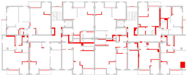
Figure 5. Wall structure of the second floor plan of the analyzed residential building in housing settlement Rasadnik; representation of the superimposed condition (planned + spontaneous) build practices
