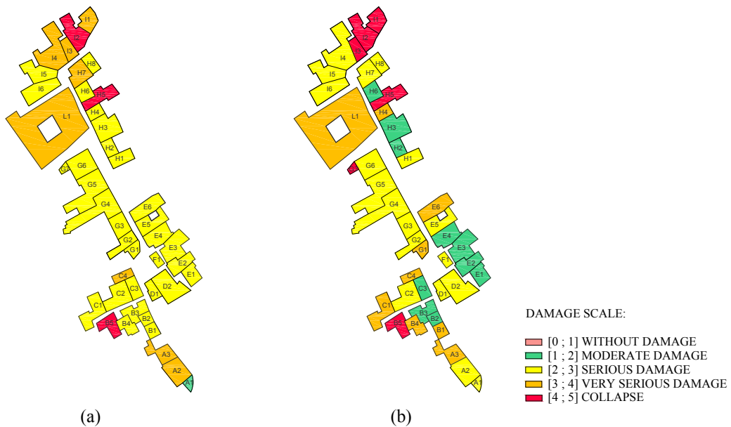
FIGURE 4. Damage maps of isolated (a) and aggregated (b) S.U. ( I_s = 12 )
