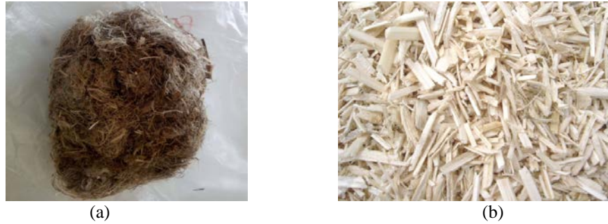
FIGURE 1. Fibres (a) and shives (b) as hemp components used in the Civil Engineering field
