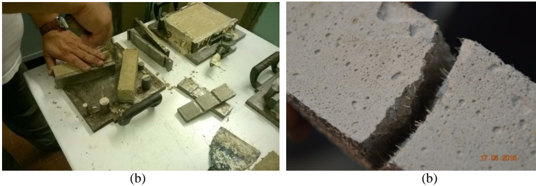
FIGURE 3. Preparation of specimens (a) and sewing effect of fibres at the bending test end (b)
