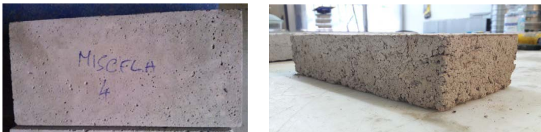
FIGURE 5. Brick specimens used for compression tests
