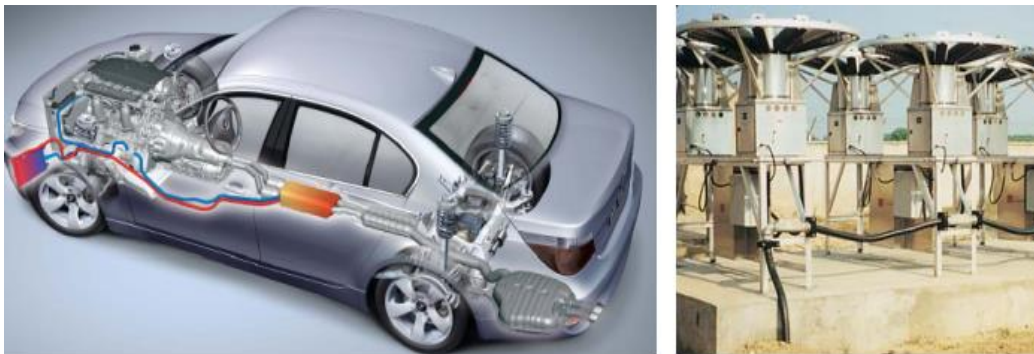
Fig. 3. 3 Waste heat recovery in vehicle (left) and TEG devices powering communications and cathodic protection of gas pipeline, India (right)
