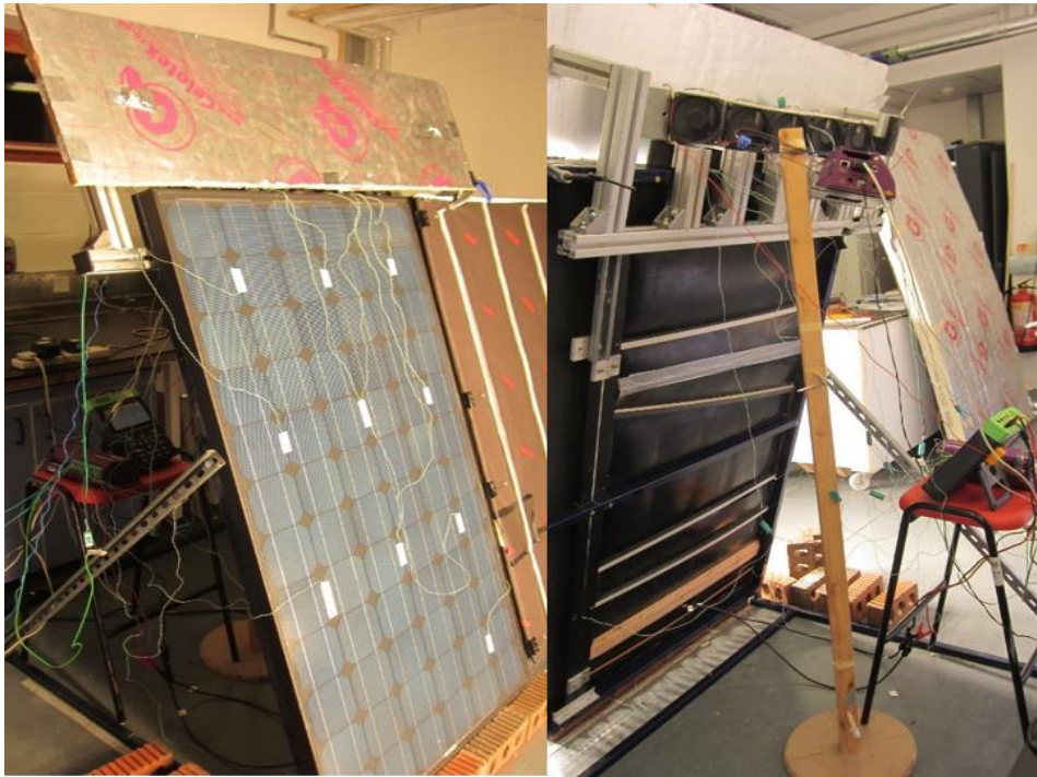
Fig. 7. 20 Photo showing tested collector and temperature sensors attached on surface as well as waste heat recovery assemblies at condenser section of heat pipe
