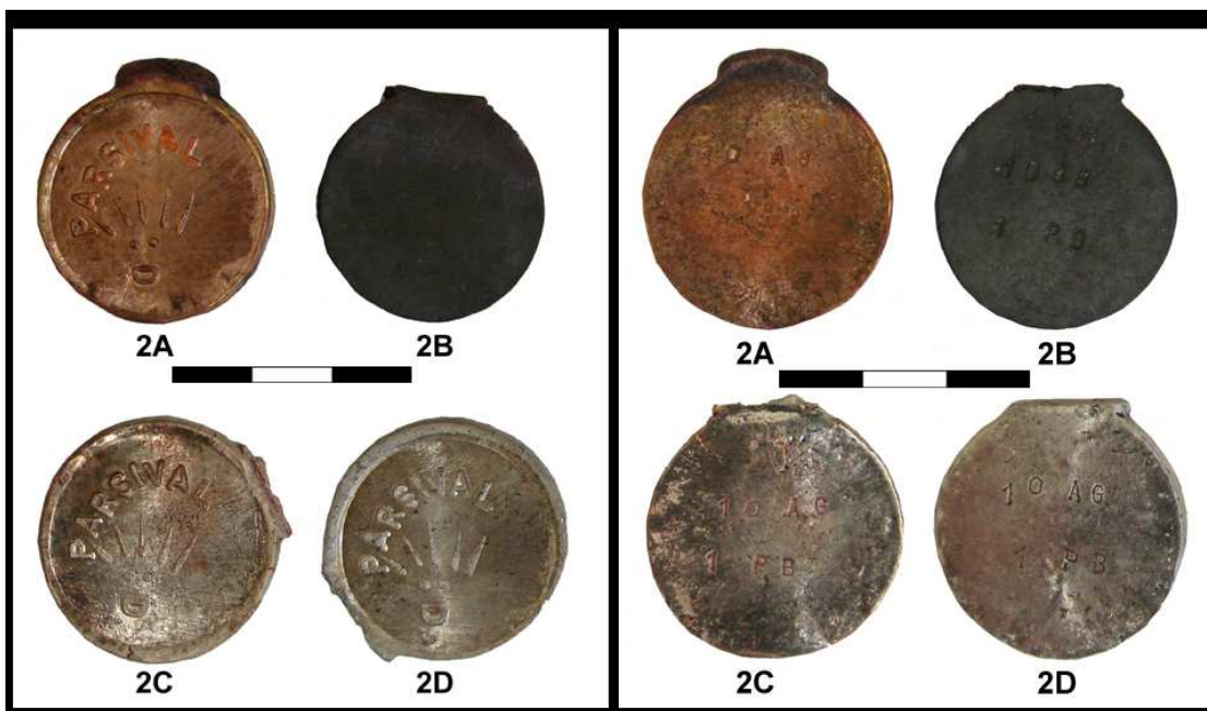
Fig. 106: Visual results (obverse and reverse) of blanks of alloy 2 (10 wt% Ag – 1 wt% Pb) after different treatments.
