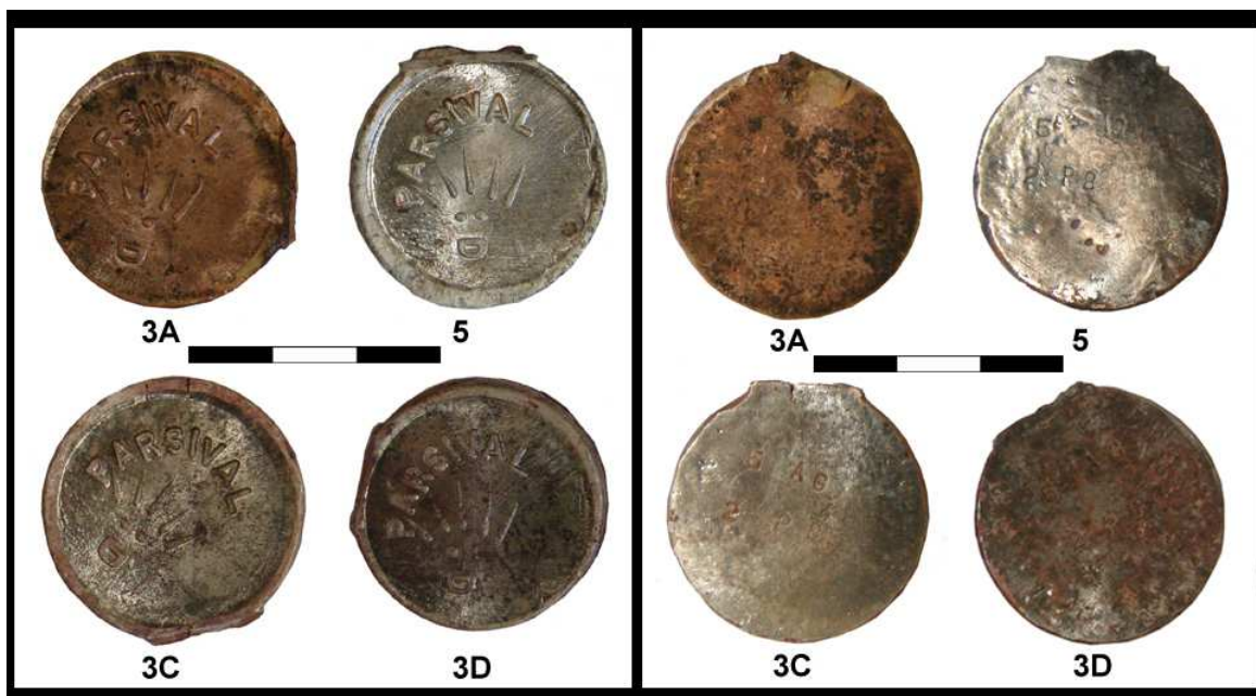
Fig. 108: Visual results (obverse and reverse) of blanks of alloy 3 (5 wt% Ag – 2 wt% Pb) after different treatments.
