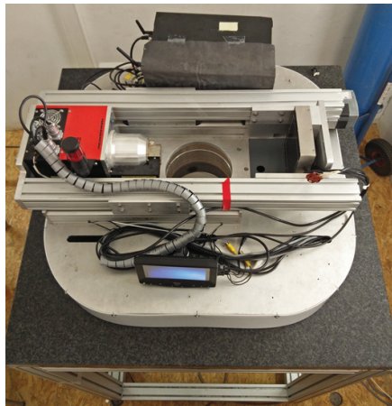
Figure 2.16: A top view on the gantry assembly of the Environmental CT scanner (EMCT), with an X-ray source on the left and a flat panel detector on the right.
