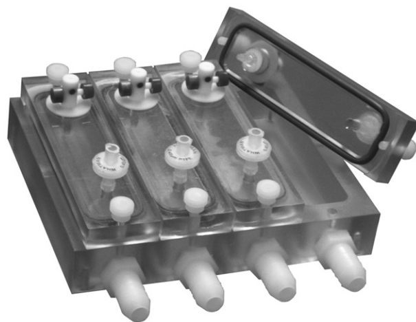
Figure 5. The Drip Flow Biofilm Reactor. Commercial version of the drip flow biofilm reactor, with four chambers each accommodating a microscope slide. © Bryan Warwood. Reuse not permitted.
