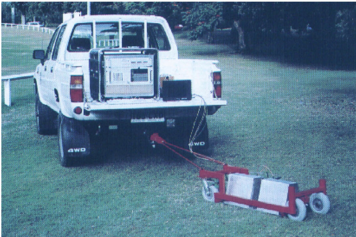
Figure 5.4: Photograph image of the 1-2 GHz SFGPR ruggedised prototype with the horn antenna trolley towed behind a 4WD
