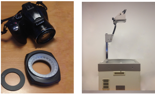
(a) Camera and macro flash ring. (b) Overhead projector as light source.
