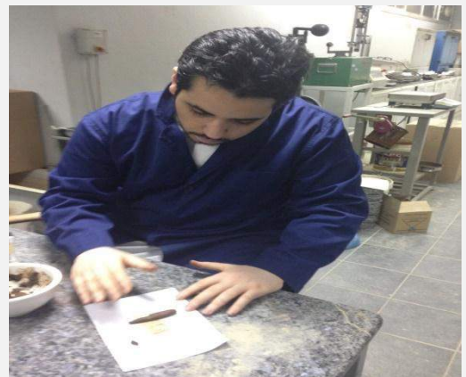
f. Shows the soil has rolled the thread between the fingers from finger-tip to the second joint of one hand and the surface of the glass rolling plate.
