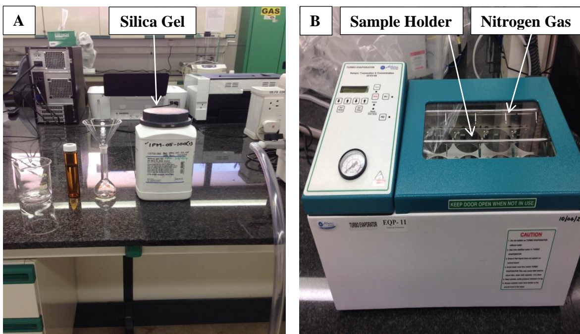
Plate 4.5. Extract sample filtration (A) and the turbo evaporation system used to concentrate the extract sample (B).
