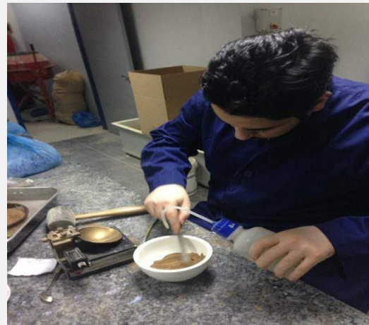
d. Show the retained soil from sieve 425 \mu\text{m} and mixed by distilled water.
