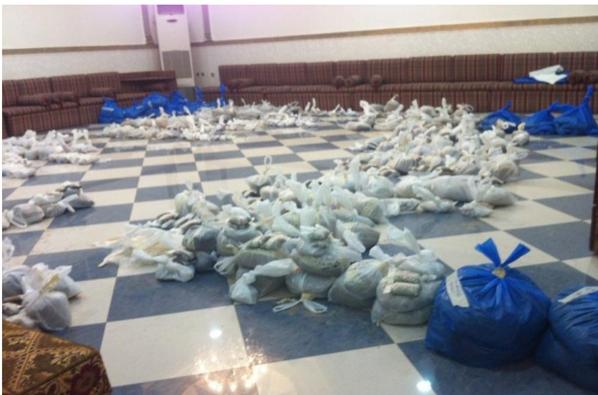
Plate 4.1. Soil samples were stored within 18 °C temperatures before transferring to the lab to be tested for Atterberg Limit, Sieve Analysis, pH and Water soluble Chloride (Cl - ) and Sulphate (SO 3 & SO 4 ) contents.
