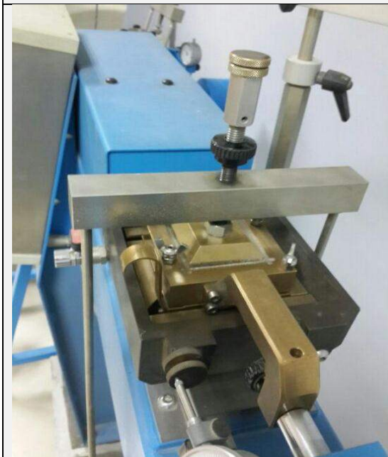
c. The Vertical load is applied and the horizontal gauge displacement is set.
