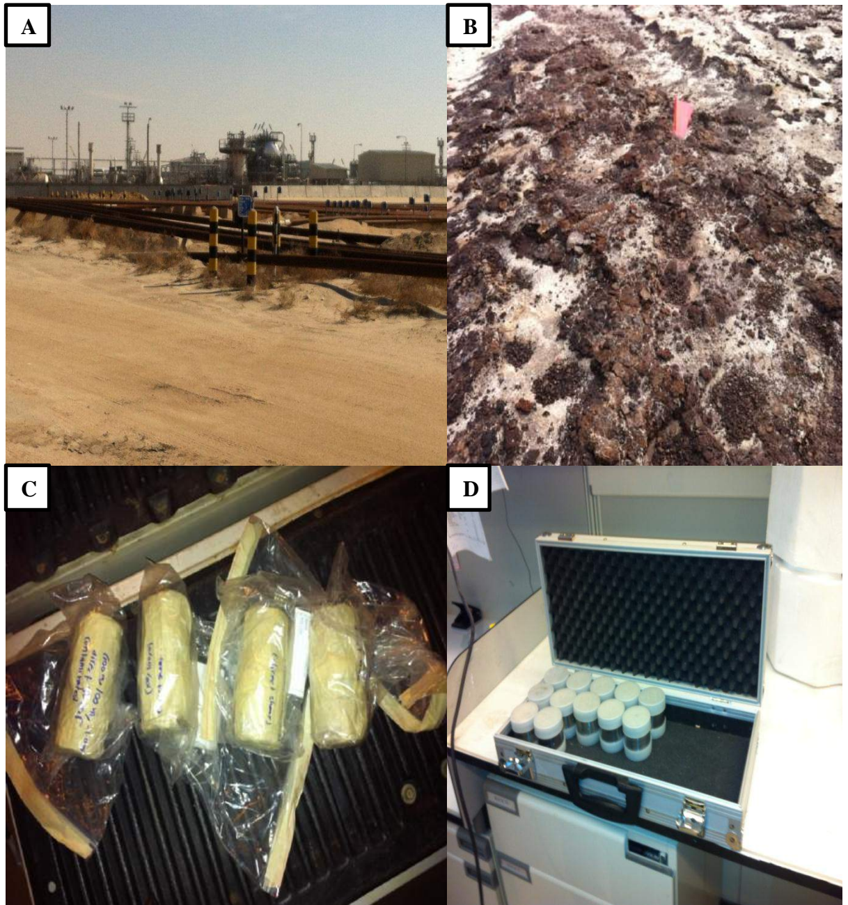
Plate A.4.2. Shows the Gas center (GC-09) close to the dry crude oil lake belong to Kuwait Oil Company (KOC) at Greater Burgan oil field (Al-Magwa Area) south west of Kuwait (A). Also, the contaminated site that is prepared with small flag in order to collect soil samples (B) as well as it shows the undisturbed contaminated soil samples for direct shear test (C) and the undisturbed contaminated soil samples for permeability test (D).
