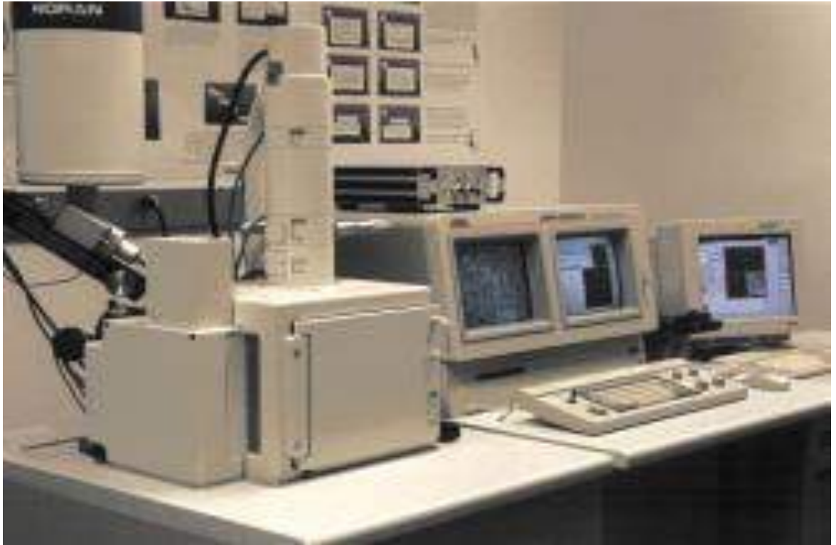
Figure A.4.17. Shows a typical SEM instrument which including the electron column, sample chamber, EDS detector, electronics console, and visual display monitors. (GIA, 2014).
