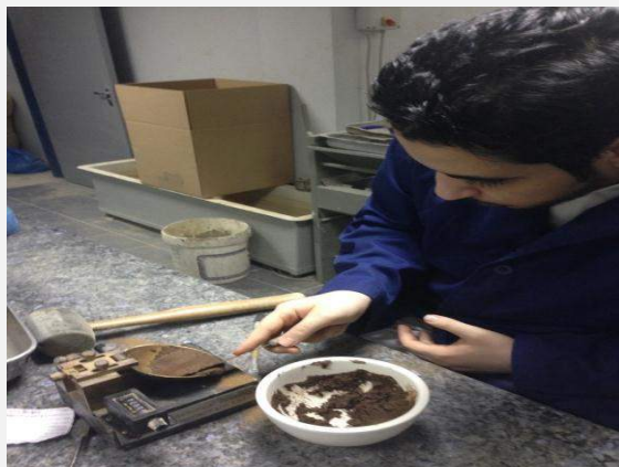
e. Shows the mixed soil sample placed in the Cup of Casagrande apparatus resting on the base.
