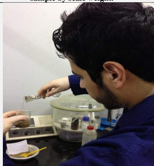
c. Shows the distil water mixing with dry soil sample.
