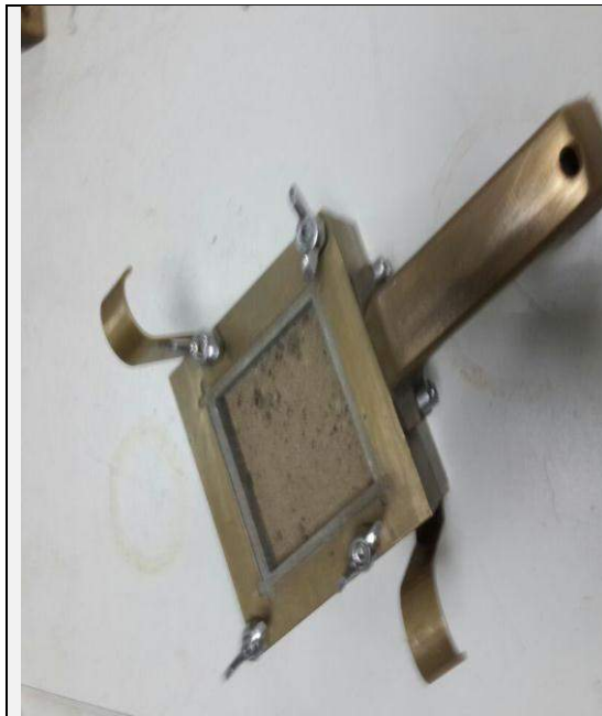
a. Showed the soil sample was tamped in the shear box (60mm square X 20 thick).
