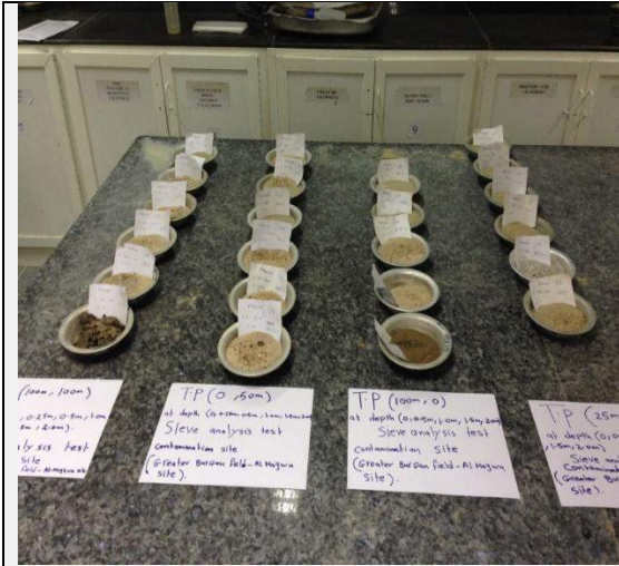
a. Shows the soil samples place to the tare
