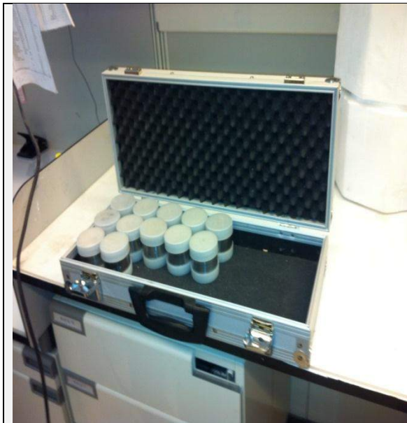
a. Collected soil samples in sampling rings.
