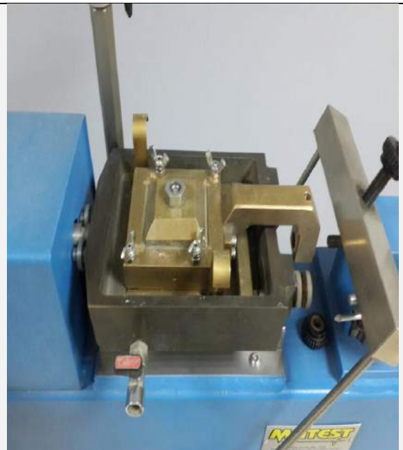
b. Shows the shear box placed in the carriage in order to apply the vertical and horizontal forces.
