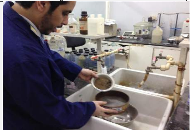
d. Shows the sample wash by distilled water.
