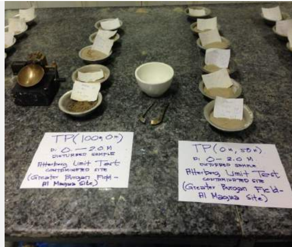
a. Shows the soil samples in tare in order to put in the oven for 24hrs.
