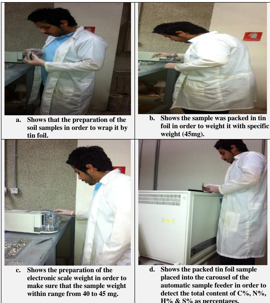
Plate A.4.9. Shows the Elemental Analyser test (Vario MACRO) in KISR lab-Ahamdai branch in Kuwait.
