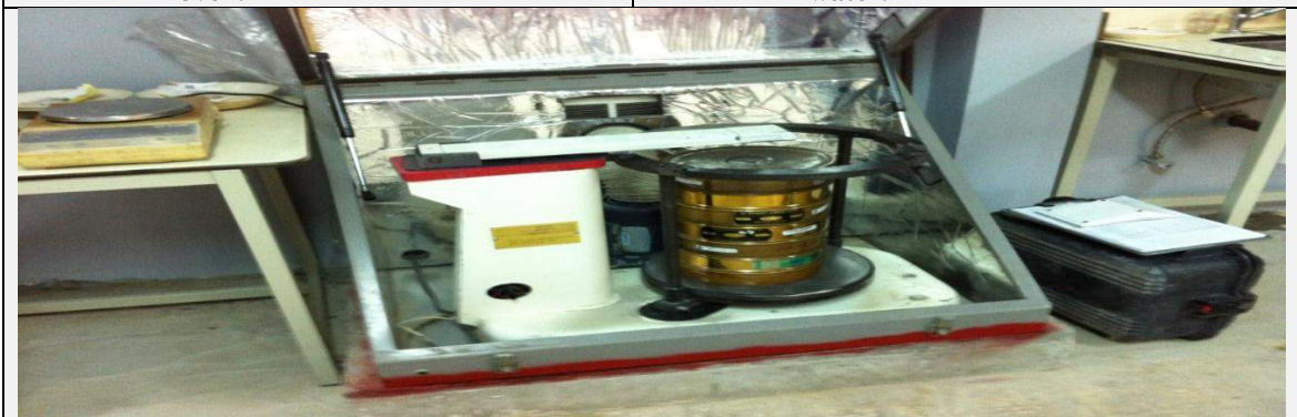
e. Shows the automatically sieve machine in order to classify the soils
