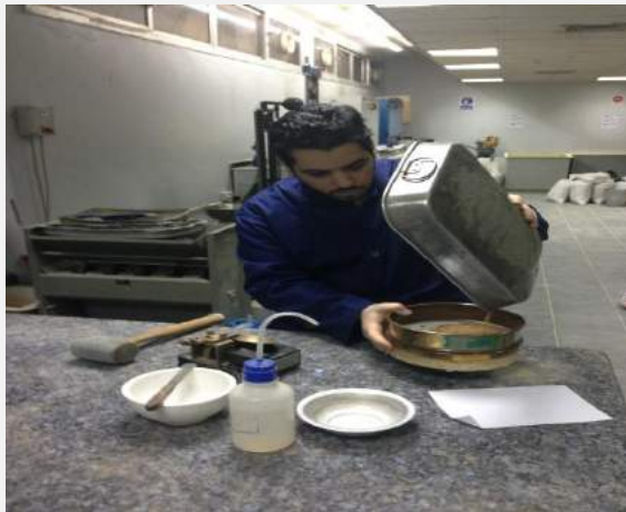
c. Shows the soil samples put it in sieve 425 \mu\text{m} in order to test the retained soil for liquid limit test.
