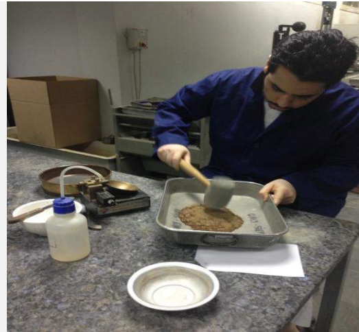
b. Shows the soil sample kibbled like powder.
