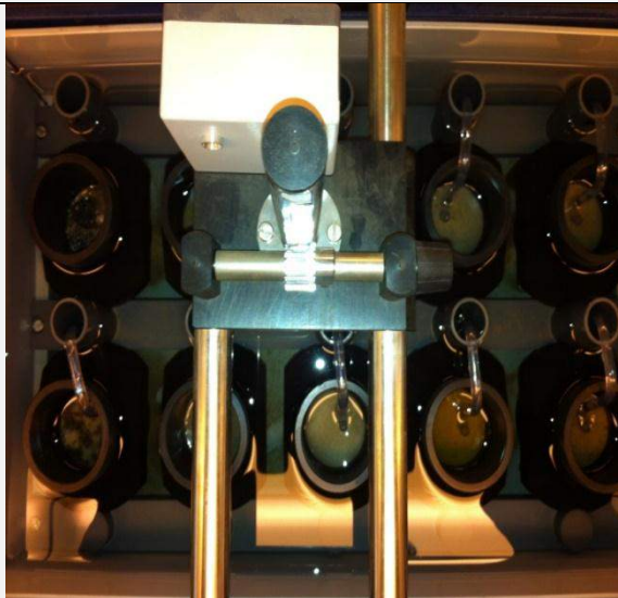
c. Soil samples the permeameter during testing.
