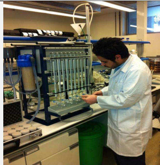
d. Measurement of volume of water during testing.
