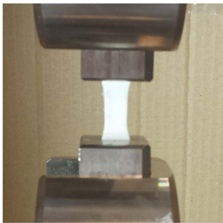
(a) Test specimen mounted in tensile test rig. The end tabs were secured directly to the test machine, and the top gripper could freely rotate to ensure no torsional forces were applied
