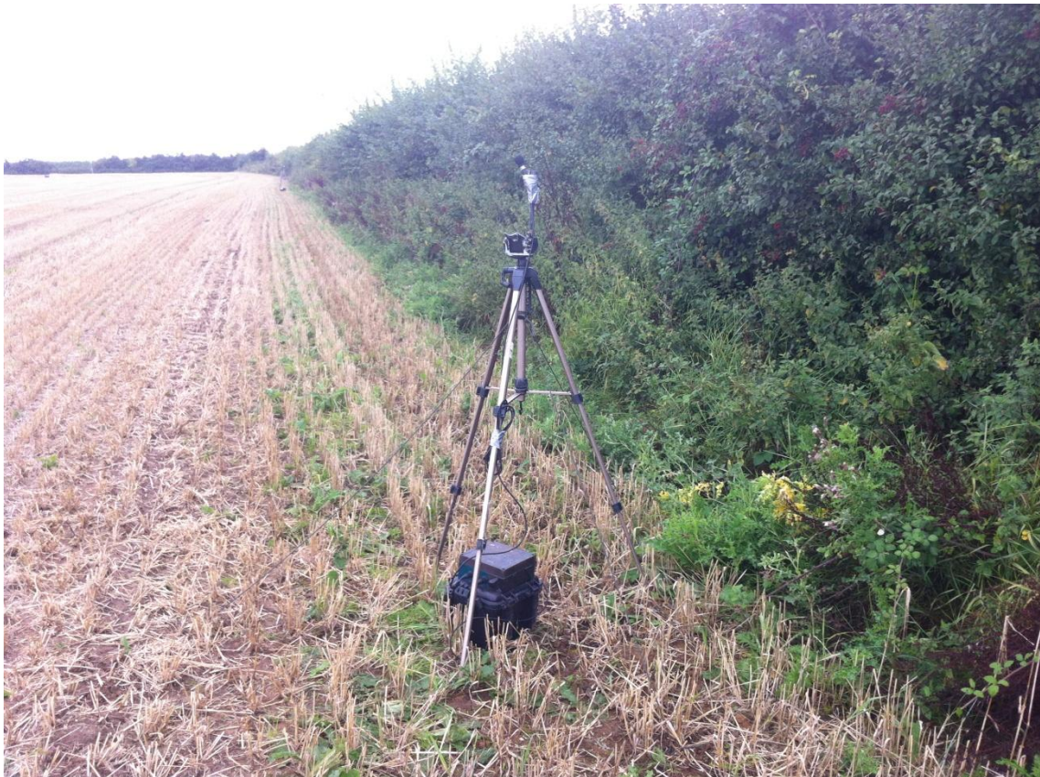
Figure 5.1: An example of an SM2 detector installed along a linear mature hedgerow during the turbine noise experiment
