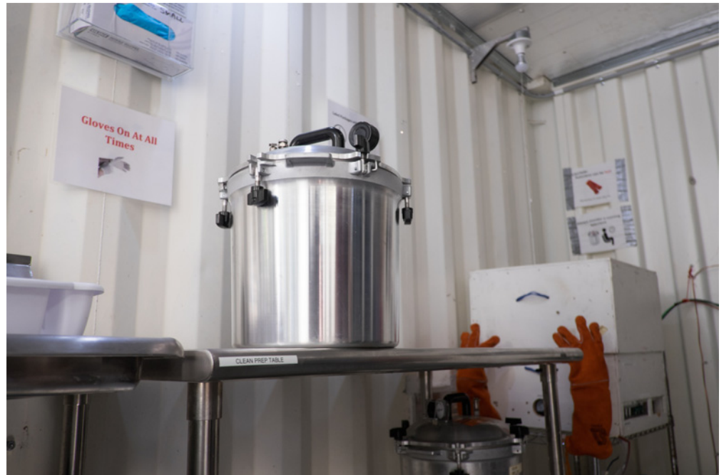
Fig 4. Non-electric steam sterilizer resting upon the preparation table.
