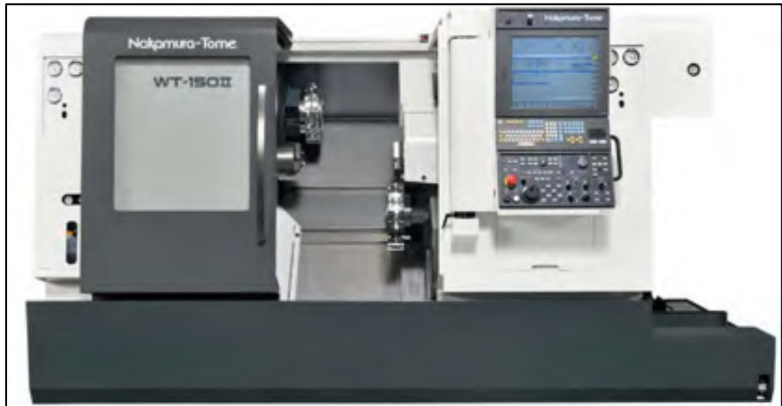
Figure 1.1 Centre de tournage-fraisage CNC Nakamura-Tome WT-150
