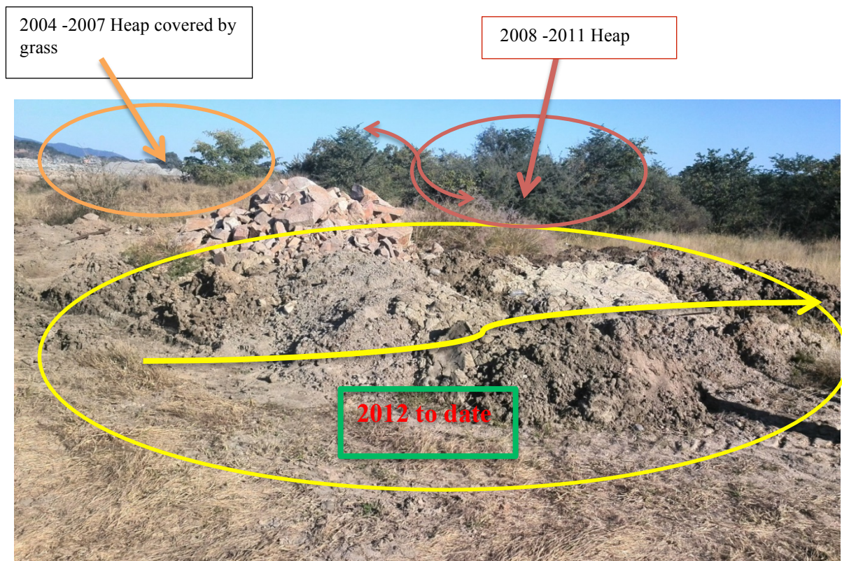
Figure 2 - Picture of different aged hydrocarbon contaminated soils stockpiles. The stockpiles were profiled according to dumping periods since the mine operations started i.e. from to 2004 to date.
