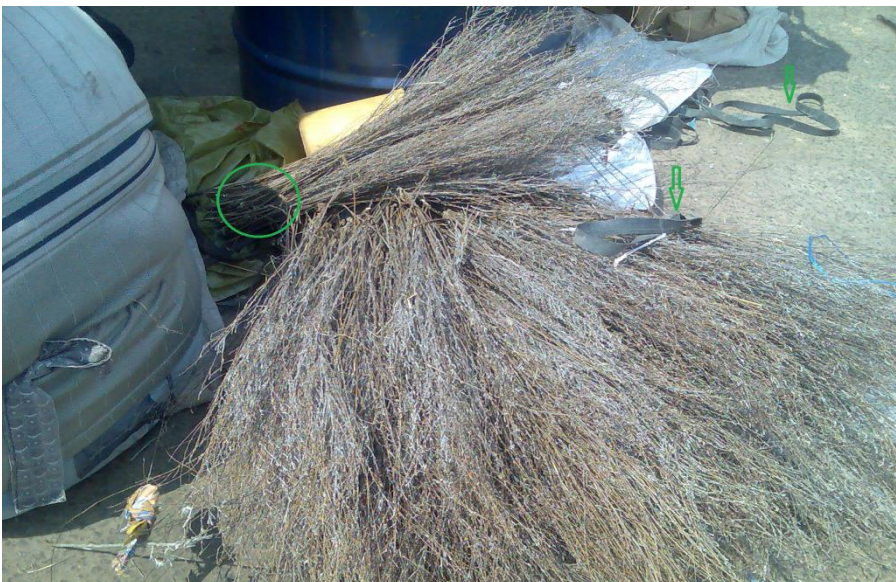
Figure 3.28: Mohlahlaila brooms being arranged to be tied with rubber bands prepared out of a tyre tube. The green arrows show the black rubber bands and the green circle identifies where the broom will be bound.
