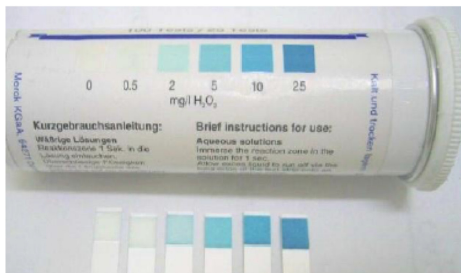
Figure 3.1 Colorimetric indication of hydrogen peroxide concentration in ROC using Merckoquant® test strips
