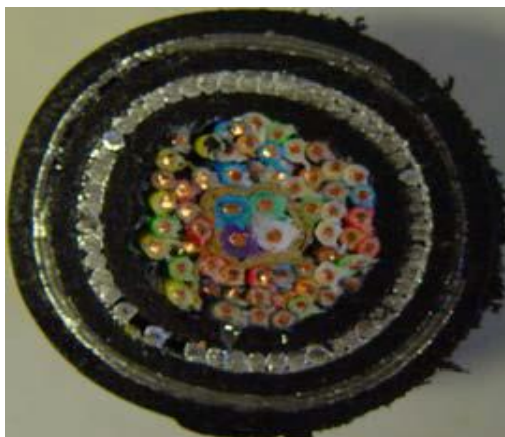
Figure 2.13: Ericsson BV-ECLALPLE 1S1.2 + 28P 0.9 cable, a typical communication cable used in the railway systems.
