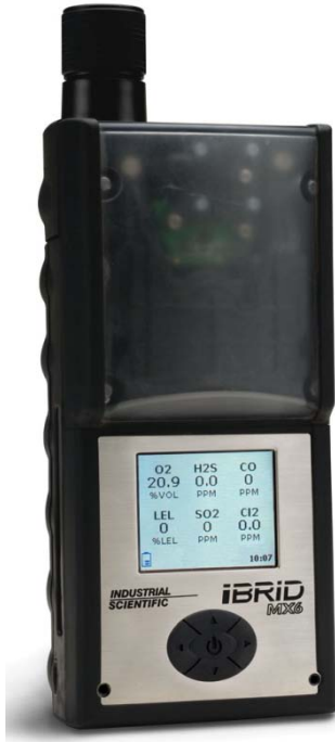
Figure 4: MX6 combustion products monitor
