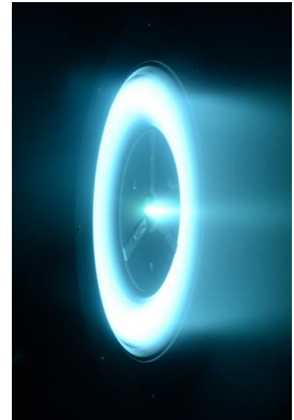
12.5 kW HERMeS operation in VF-5 at GRC
