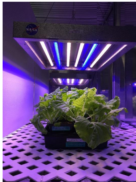
Figure 3. White plus discrete LEDs used to study growth of lettuce and Chinese cabbage.
