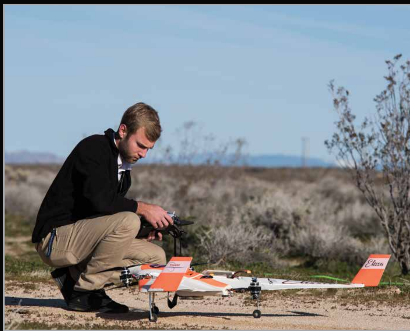
Jacobs Technology Inc. safety pilot Alex Flock pre-flights Elissa, NASA Armstrong's autonomy testbed.
