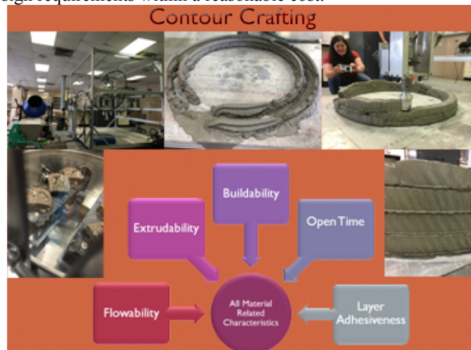
Figure 1. Some of the Main Challenges for the Concrete Contour Crafting.
