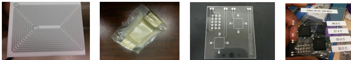
Figure 4. A few functional parts Aerosol Jet ® printed by MSFC Additive Electronics Lab
