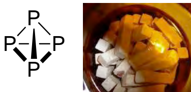
Figure IV-1. White phosphorus (P 4 ), in its structural formula (left) and in its physical form (right).
