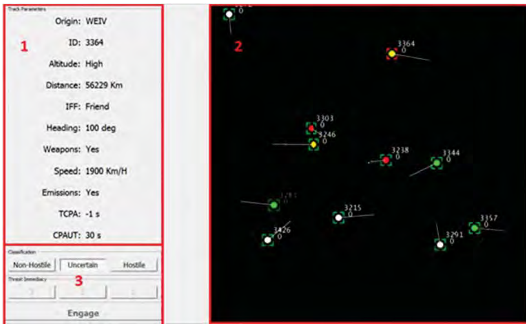
Figure 54.: Screenshot of S-CCS visual interface divided into three areas: 1) a list providing information on a number of parameters about the selected aircraft; 2) a radar display depicting in real-time all aircraft moving at various speeds and trajectories around the ship (central point) and 3) a set of classification buttons allowing the participants to allocate threat level and immediacy to an aircraft and to engage with missile fire a hostile candidate.
