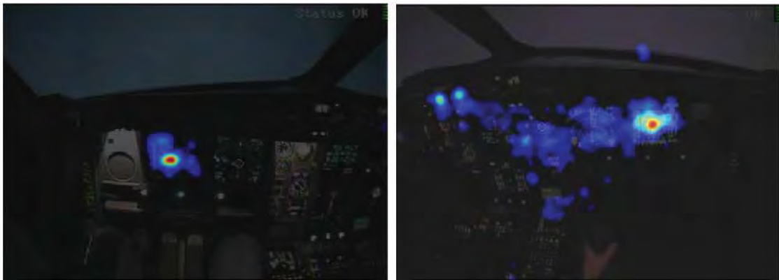
Figure 48.: Attentional maps during go-around for pilot flying (on the left) and pilot monitoring (on the right).
