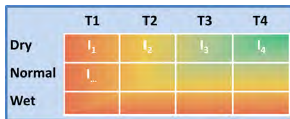
FIGURE A.4 – A possible example of the flash flood forecasting diagram via the FFG method. The threshold intensity is given for various forecast lead times ( T_1, T_2, \dots ) and different initial wetness conditions (Dry, Normal, Wet).
