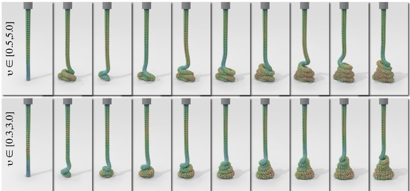
Fig. 8. Jet buckling with different viscosity intervals. Our method provides different coiling effects varying the parameters of Cross model.
