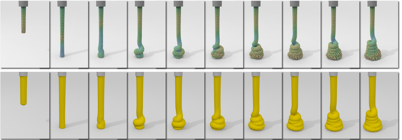
Fig. 6. The formation of coils in a falling stream of viscous liquid.
