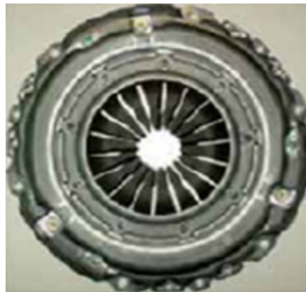
Figure 2.8 : Push type clutch [11].
