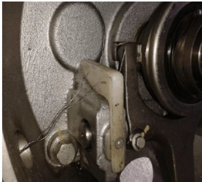
Figure 4.8 : Thermocouple position near clutch release bearing.
