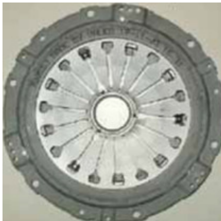
Figure 2.10 : Pull type clutch [11].
