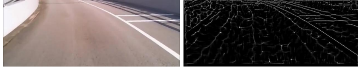
Figure 2.3: Original image and grey-scale image based on ridgeness value
