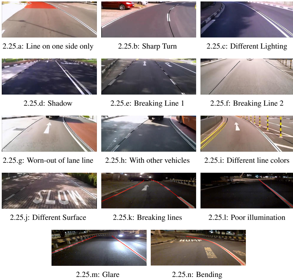
Figure 2.25: Fitting results under different situations. a \sim j daytime vision (black line) and k \sim n night vision (red line)
