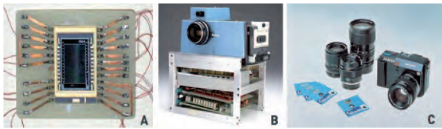
Fig. 2. (A) One of the earliest CCD devices from Bell Labs. (B) Kodak camera. (C) Sony Mavica camera.
