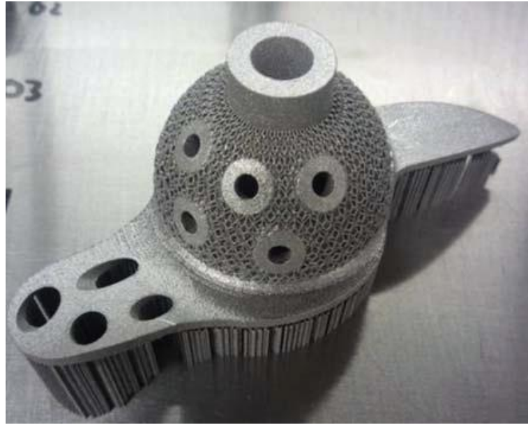
Figure 2.8. Additive manufactured hip endoprosthesis fabricated by a selective laser melting process [44]
