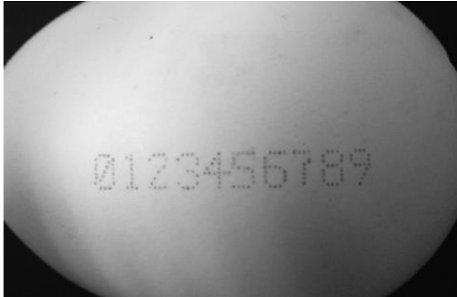
Figure 2.17. Example identification characters laser marked directly the shell of an egg [66]
