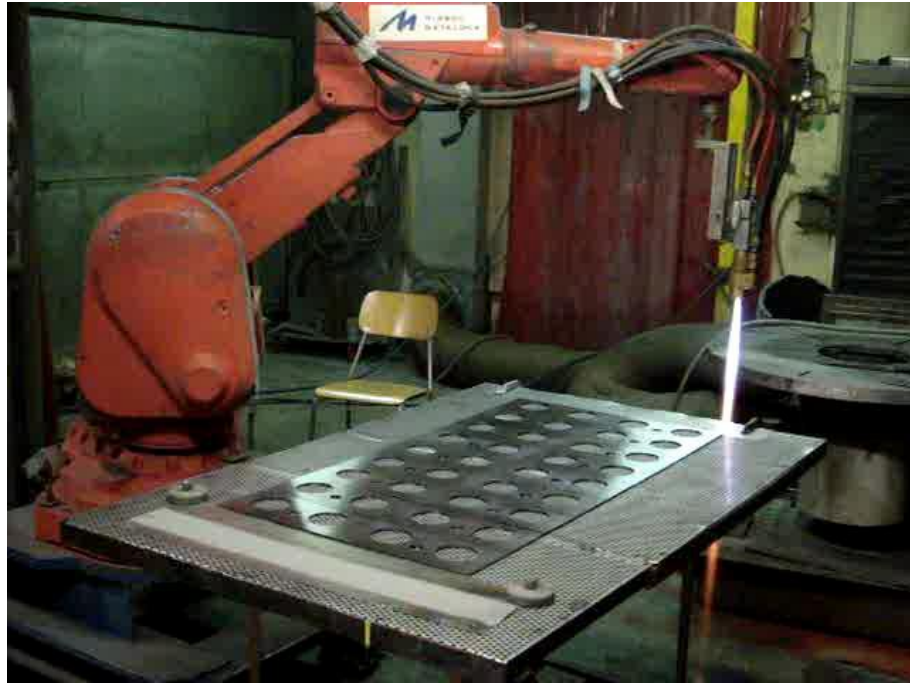
Figure 2.6. Photograph of a robotic arm HVOF spraying of steel shims for MDT
