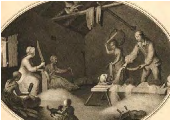
Figure 203 Hincks, W. (1791) Irish linen industry -The common method of Beetling, Scutching, and Hackling the Flax, Plate 4. [stipple, etching on paper] London: British Museum 1877,0113.373
