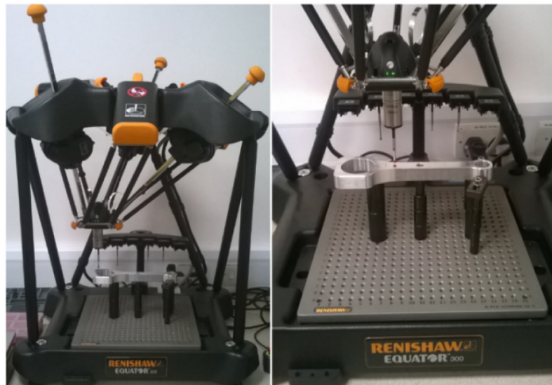
Fig. 8. Test setup on Renishaw Equator for preliminary experiments.
