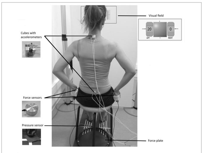
FIGURE 1 | Experimental set-up with the subject applying a unilateral compressive load at 20% of the maximum voluntary contraction (MVC).
