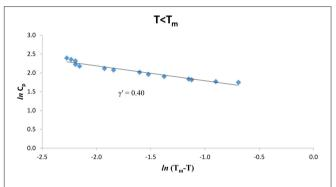
FIGURE 1 | InC<sub>p</sub> against In( $T_m$  – T) for  $T < T_m$  according to Equation (2) for pure CH<sub>4</sub> using the experimental data [8].
