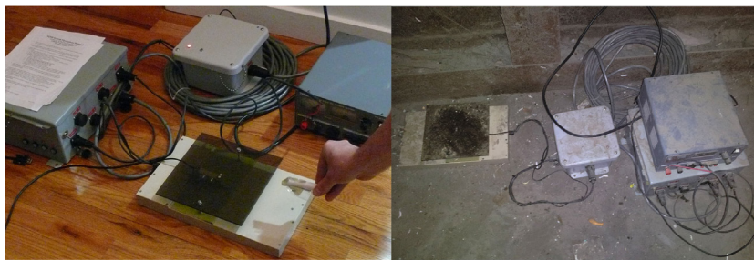
FIGURE 2 | RFID system. Sensor, data logger, system control unit.
