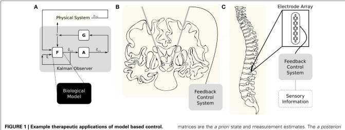
(A) The system dynamics are described by a model, F, and the observations are described by a function, A. In most systems those observations are going to be noisy, so a covariance matrix, R, will account for that. After one step of F, using the resulting sigma points will provide  $\tilde{X}_i = F(X_i)$ . A new set of observations can then be found,  $\tilde{Y}_i = A(X_i)$ . The means over these two
