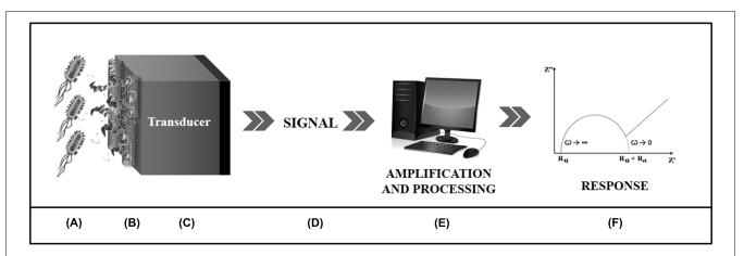
FIGURE 2 | Schematic presentation of an electrochemical biosensor. The detection of the analyte (A) is performed through a biological component (B) associated to a transducer (C). This is responsible for converting the
