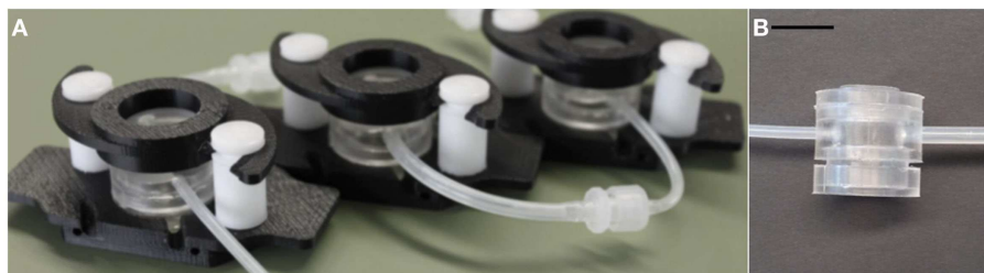
FIGURE 1 | (A) Example of a MCmB circuit with three chambers, (B) A single MCmB module. Scale bar represents 10 mm.
